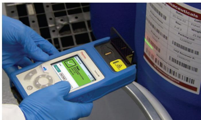
engine collects not just the sample spectrum but also the measurement uncertainty at the moment of analysis, which allows the analyzer to adaptively adjust collection parameters to a wide variety of potential interferences (such as lighting, temperature and operator usage).
